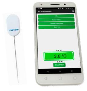
The Metos IoLiving I sensor allows temperatures to be measured in situations like a lunch table, goods reception inspection etc.
